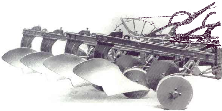
Side View of Old Abe—Note the height to which bottoms are raised
